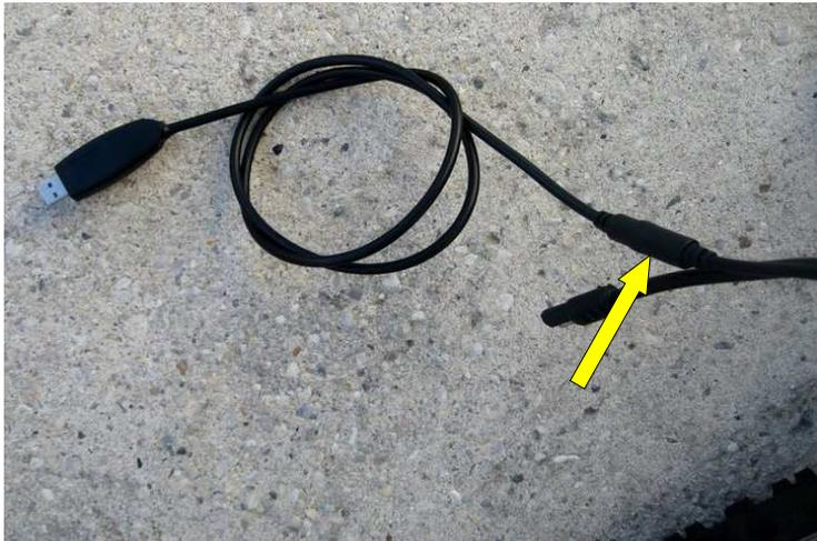
Connect the black plastic connector of the programming cable in the space of the existing one, the one used to connect the throttle.
