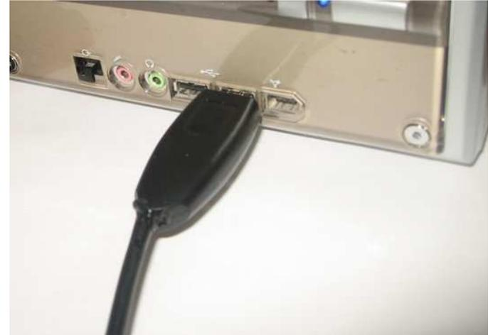
Connect the USB plug of the programming cable on the USB port of your PC.
