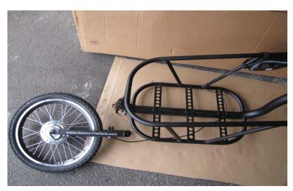
Turn around the trailer and fix the fork on the central axis of the frame :
