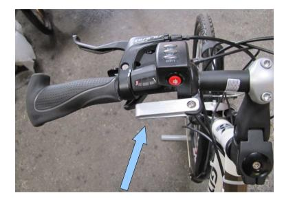
On this picture, we have put an extension (in aluminium) to make access easier.
