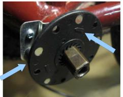
Put the washer holding the magnets on the chainset axis.
