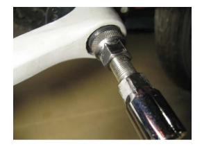
Screw the **crank extractor** then remove the crank
