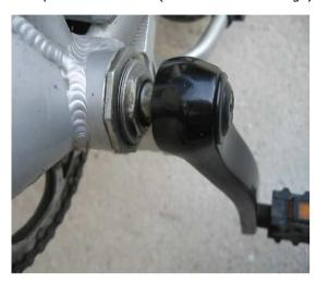
• Example of incompatible chainset (with external bearings) :
