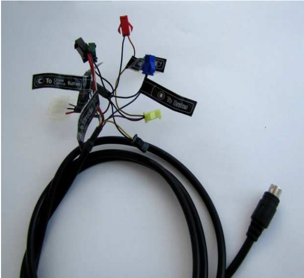
Main cable of connection of the accessories with its colored connectors
