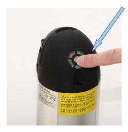
On the contrary, during the **charge** of the battery, the **green lights switch on** until they are **all on.**
