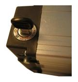
At this point, the battery is on and fixed to the sliding rack. You can not remove the key, the battery is safely fastened to the rack and the vehicle is ready to go.
