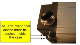
At this point, the battery is turned off and fixed to the sliding rack. You can **remove** the key, the battery is safely fastened to the rack.
